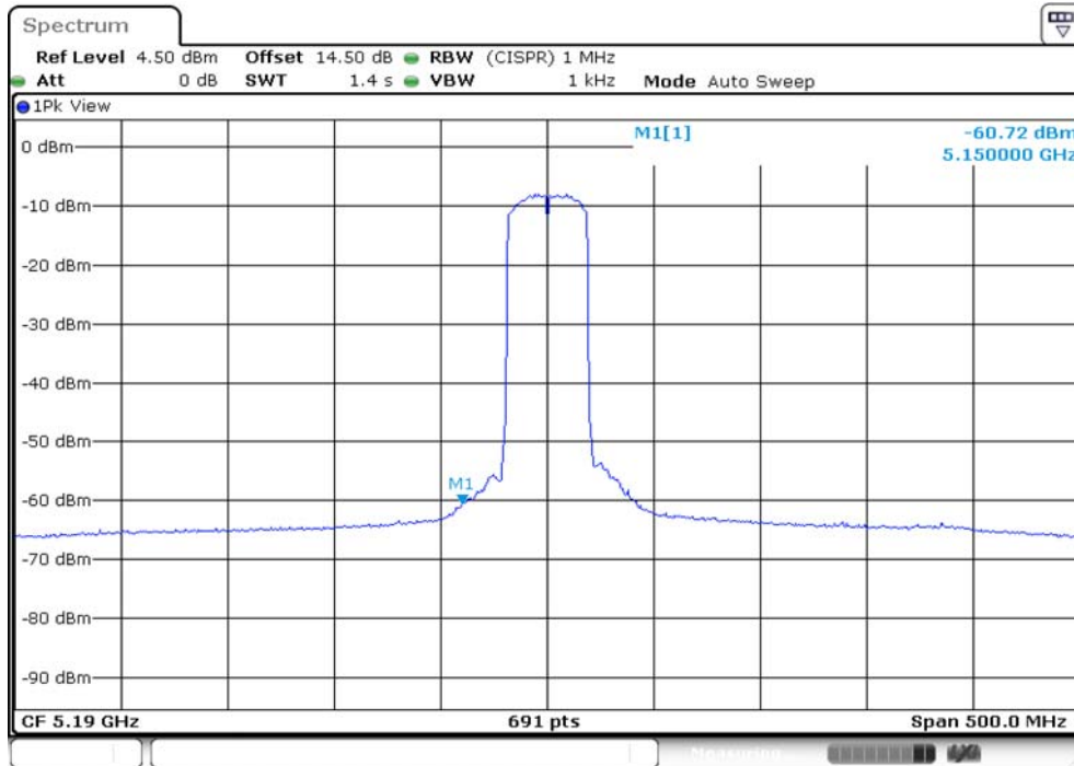
Plot on IEEE 802.11ac Nss1 MCS0 VHT40 / 5190 MHz / Average / Port 2
