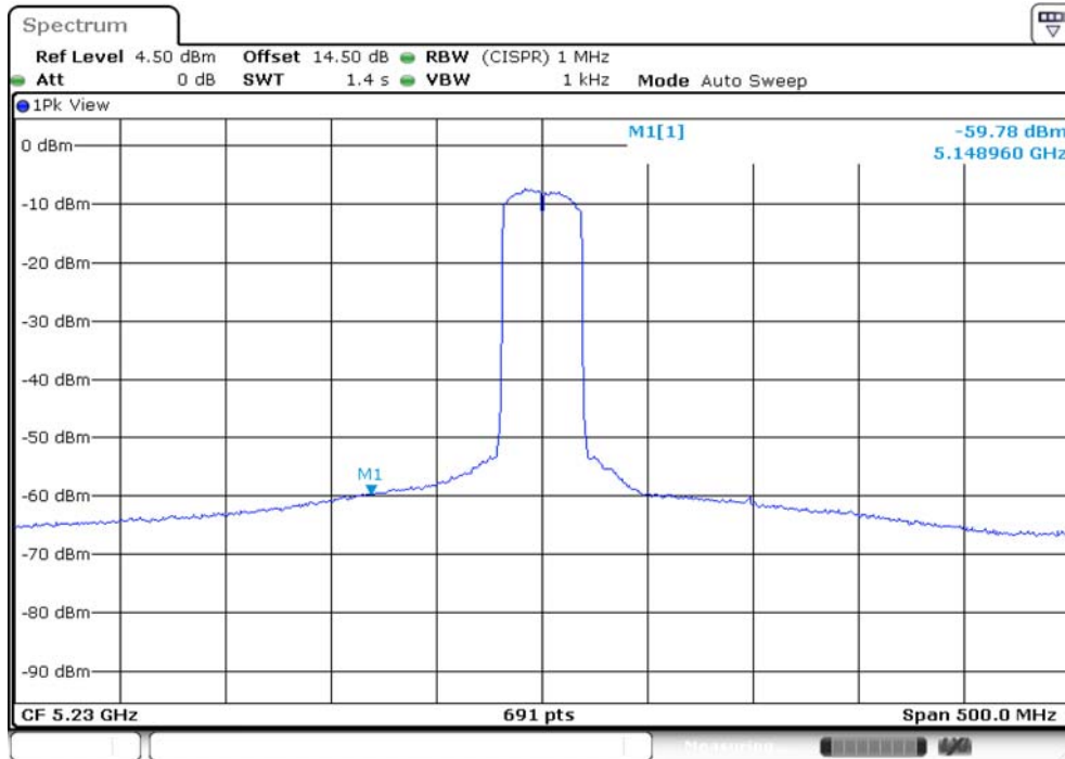
Plot on IEEE 802.11ac Nss1 MCS0 VHT40 / 5230 MHz / Average / Port 2
