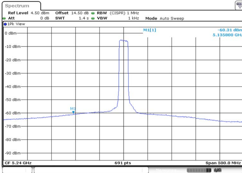
Plot on IEEE 802.11ac Nss1 MCS0 VHT20 / 5240 MHz / Average / Port 2
