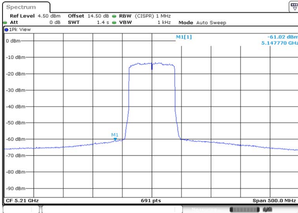
Plot on IEEE 802.11ac Nss1 MCS0 VHT80 / 5210 MHz / Average / Port 2
