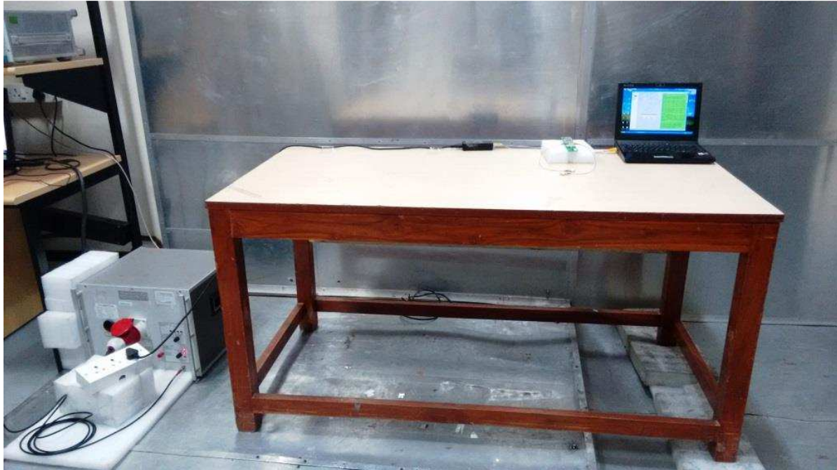
Figure 13: Conducted Emission Test set up photograph – 150 kHz to 30 MHz
