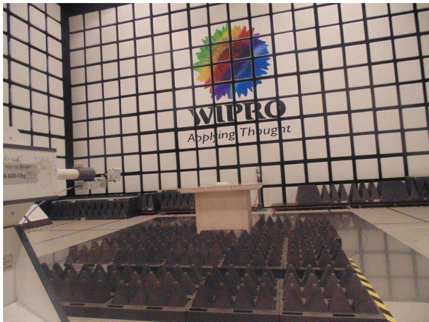
Figure 10: Test setup for Radiated Emission Test from 18 GHz to 40 GHz – Horizontal Polarization
