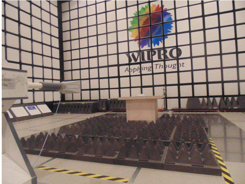
Figure 9: Test setup for Radiated Emission Test from 1 GHz to 18 GHz – Vertical Polarization
