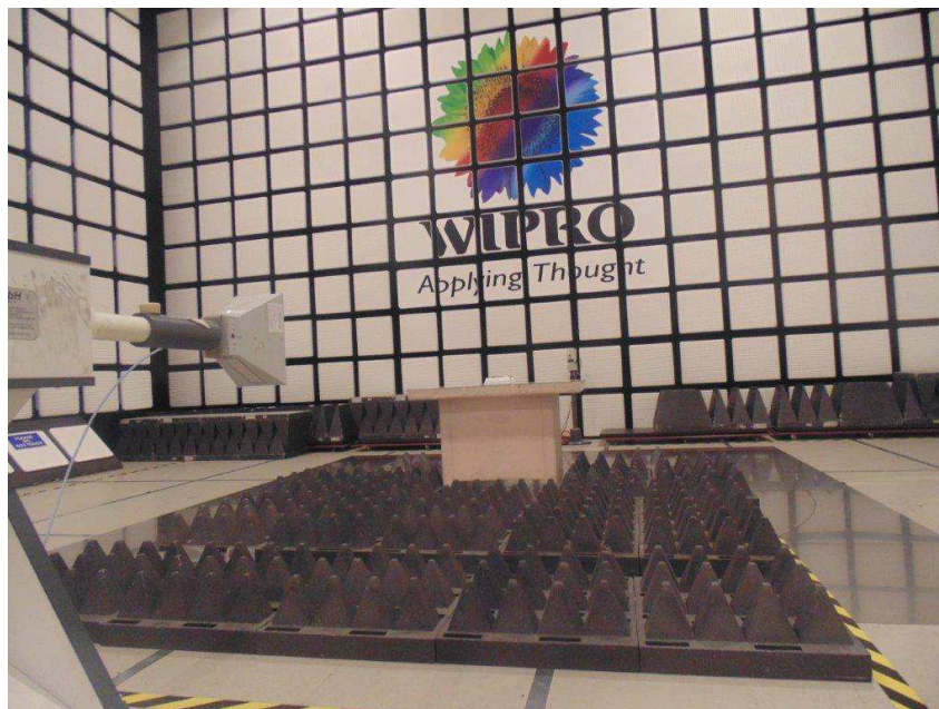
Figure 8: Test setup for Radiated Emission Test from 1 GHz to 18 GHz - Horizontal Polarization
