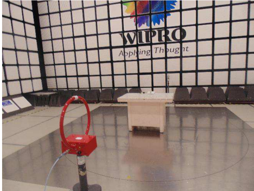
Figure 5: Test setup for Radiated Emission E field measurement from 9 kHz to 30MHz
