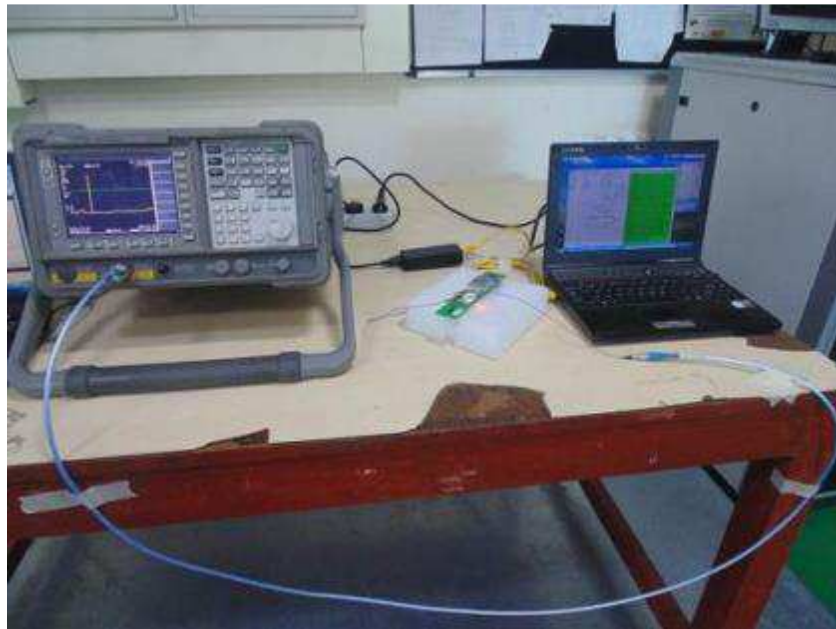
Figure 14: Conducted RF Test set up photograph
