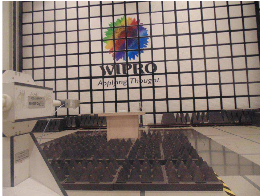
Figure 11: Test setup for Radiated Emission Test from 18 GHz to 40 GHz – Vertical Polarization
