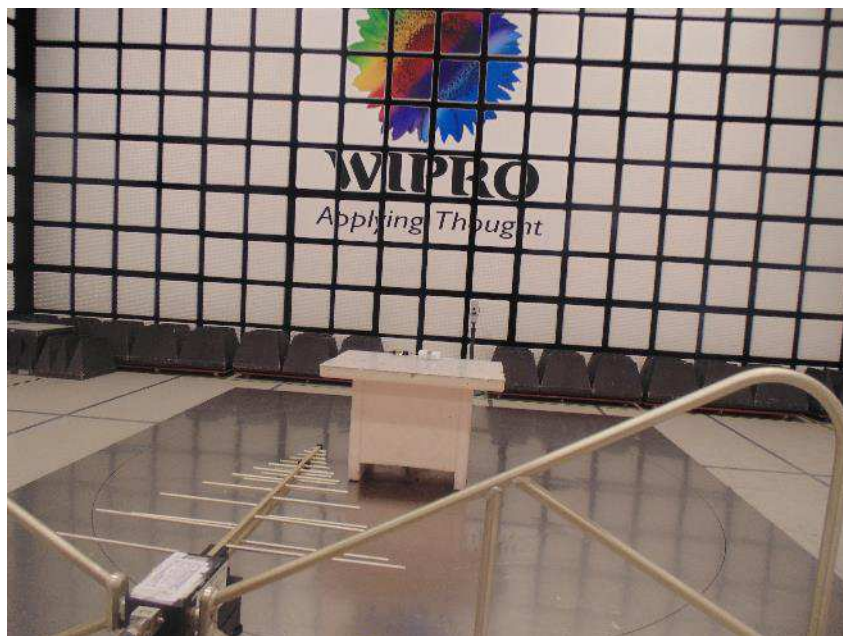
Figure 6: Test setup for Radiated Emission test from 30MHz to 1GHz - Horizontal Polarization
