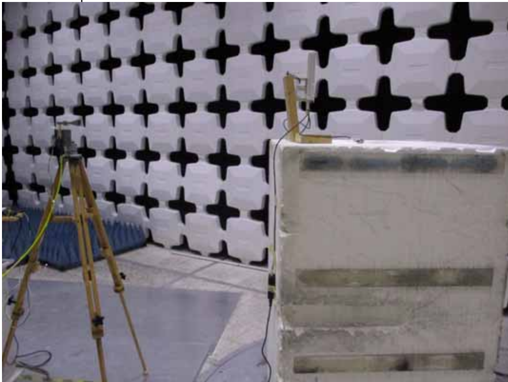
Test Setup for Radiated Emissions above 18-26.5GHz – Vertical Polarization
