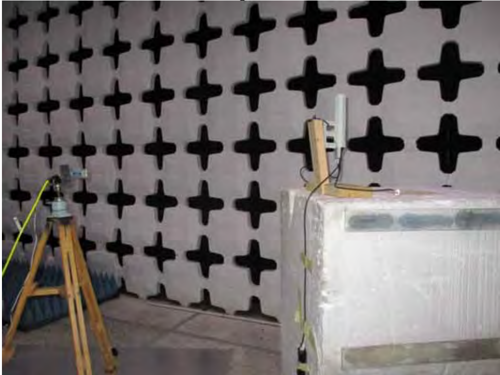
Test Setup for Radiated Emissions above 18-26.5GHz – Horizontal Polarization
