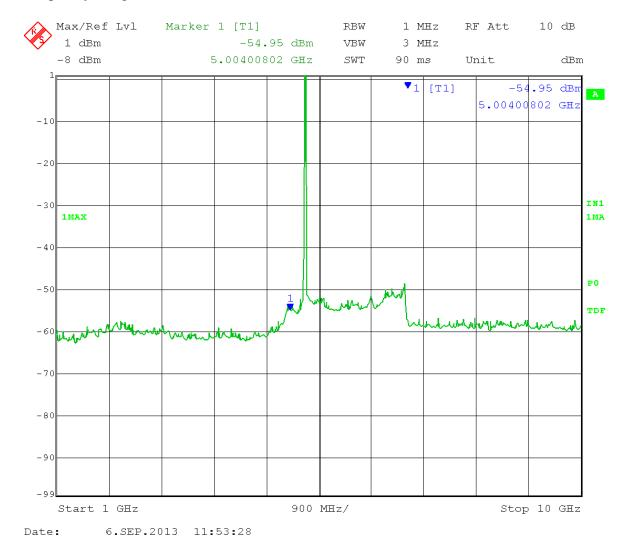
Marker 1: Calculated Field Strength (Restricted Band) = -54.95 + 16dBi antenna gain + 3 dB (MIMO) - 20 log (3 meters) + 104.77 = 59.28dB $\mu$ V/m Peak
