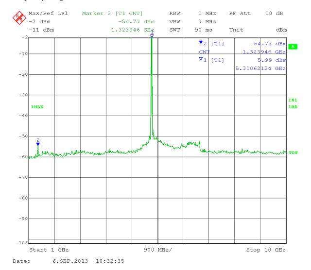
Marker 2: Calculated Field Strength (Restricted Band) = -54.73 + 16dBi antenna gain + 3 dB (MIMO) - 20 log (3 meters) + 104.77 = 59.5dB $\mu$ V/m Peak
