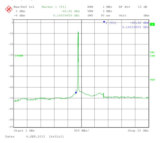
Marker 1: Calculated Field Strength (Restricted Band) = -65.92 + 16dBi antenna gain + 3 dB (MIMO) - 20 log (3 meters) + 104.77 = 48.31dB $\mu$ V/m Peak
