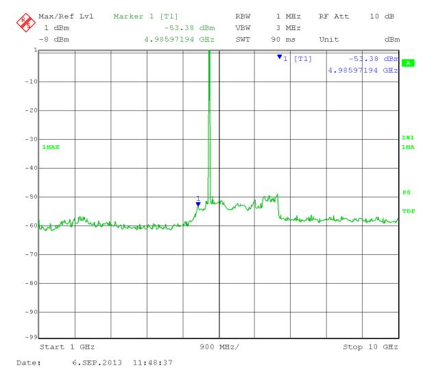
Marker 1: Calculated Field Strength (Restricted Band) = -53.38 + 16dBi antenna gain + 3 dB (MIMO) – 20 log (3 meters) + 104.77 = 61.45dB $\mu$ V/m Peak
