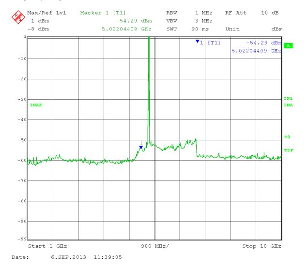
Marker 1: Calculated Field Strength (Restricted Band) = -54.29 + 16dBi antenna gain + 3 dB (MIMO) - 20 log (3 meters) + 104.77 = 59.94dB $\mu$ V/m Peak
