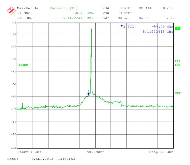
Marker 1: Calculated Field Strength (Restricted Band) = -58.70 + 16dBi antenna gain + 3 dB (MIMO) – 20 log (3 meters) + 104.77 = 55.53dB $\mu$ V/m Peak
