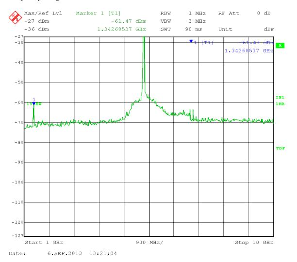
Marker 1: Calculated Field Strength (Restricted Band) = -61.47 + 16dBi antenna gain + 3 dB (MIMO) - 20 log (3 meters) + 104.77 = 52.76dB $\mu$ V/m Peak
