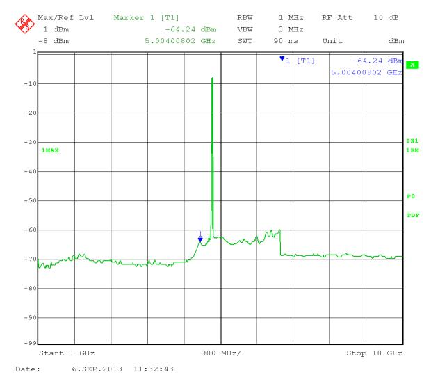
Marker 1: Calculated Field Strength (Restricted Band) = -64.24 + 16dBi antenna gain + 3 dB (MIMO) - 20 log (3 meters) + 104.77 = 49.99dB $\mu$ V/m Average
