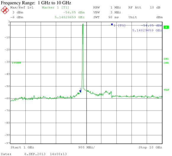
Marker 1: Calculated Field Strength (Restricted Band) = -54.85 + 16dBi antenna gain + 3 dB (MIMO) - 20 log (3 meters) + 104.77 = 59.38dB $\mu$ V/m Peak
