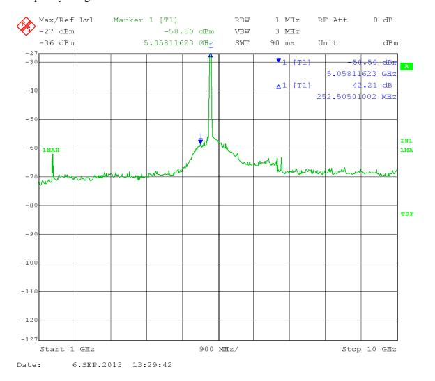
Marker 1: Calculated Field Strength (Restricted Band) = -58.50 + 16dBi antenna gain + 3 dB (MIMO) - 20 log (3 meters) + 104.77 = 55.73dB $\mu$ V/m Peak
