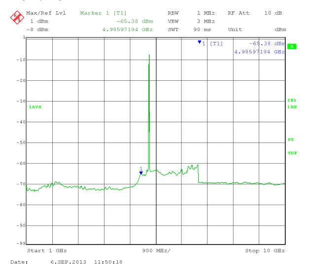
Marker 1: Calculated Field Strength (Restricted Band) = -65.38 + 16dBi antenna gain + 3 dB (MIMO) - 20 log (3 meters) + 104.77 = 48.85dB $\mu$ V/m Average
