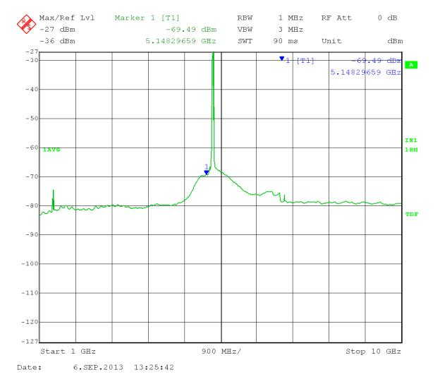
Marker 1: Calculated Field Strength (Restricted Band) = -69.49 + 16dBi antenna gain + 3 dB (MIMO) - 20 log (3 meters) + 104.77 = 44.74dB $\mu$ V/m Peak
