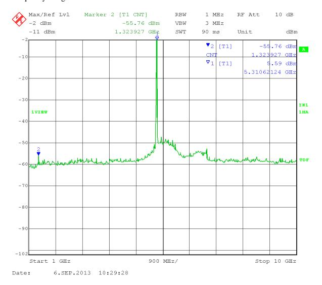
Marker 2: Calculated Field Strength (Restricted Band) = -55.76 + 16dBi antenna gain + 3 dB (MIMO) - 20 log (3 meters) + 104.77 = 58.47dB $\mu$ V/m Peak
