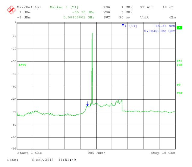
Marker 1: Calculated Field Strength (Restricted Band) = -65.36 + 16dBi antenna gain + 3 dB (MIMO) – 20 log (3 meters) + 104.77 = 48.87dB $\mu$ V/m Average
