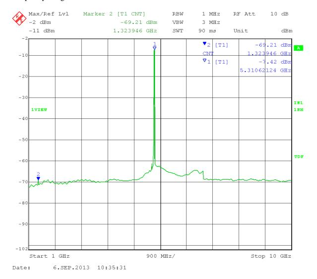
Marker 2: Calculated Field Strength (Restricted Band) = -69.21 + 16dBi antenna gain + 3 dB (MIMO) - 20 log (3 meters) + 104.77 = 45.02dB $\mu$ V/m Average
