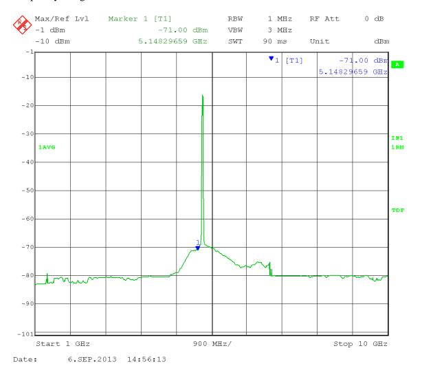
Marker 1: Calculated Field Strength (Restricted Band) = -71.00 + 16dBi antenna gain + 3 dB (MIMO) – 20 log (3 meters) + 104.77 = 43.23dB $\mu$ V/m Peak
