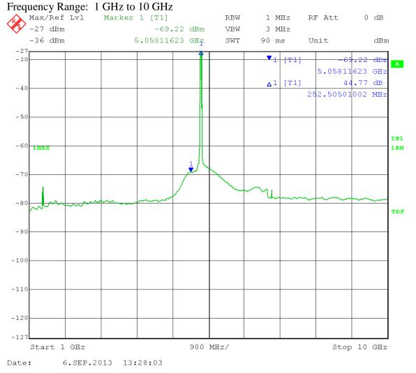
Marker 1: Calculated Field Strength (Restricted Band) = -69.20 + 16dBi antenna gain + 3 dB (MIMO) - 20 log (3 meters) + 104.77 = 45.03dB $\mu$ V/m Peak
