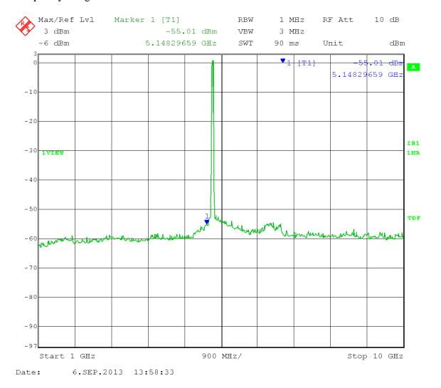
Marker 1: Calculated Field Strength (Restricted Band) = -55.01 + 16dBi antenna gain + 3 dB (MIMO) – 20 log (3 meters) + 104.77 = 59.22dB $\mu$ V/m Peak
