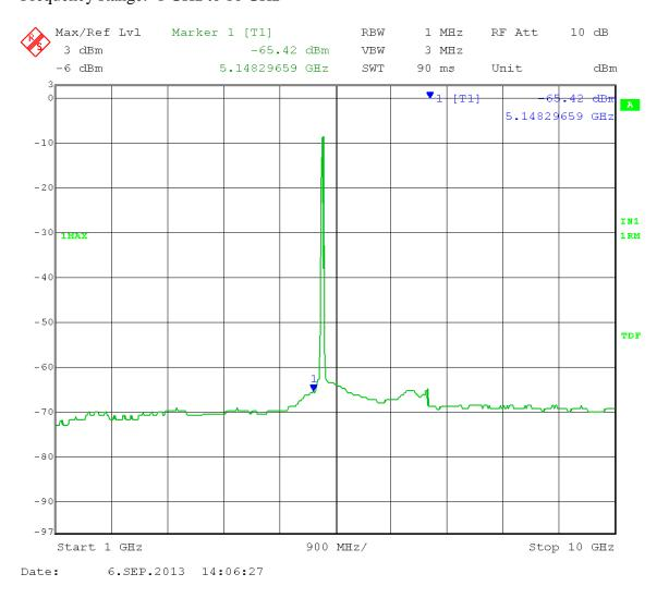
Marker 1: Calculated Field Strength (Restricted Band) = -65.42 + 16dBi antenna gain + 3 dB (MIMO) - 20 log (3 meters) + 104.77 = 48.81dB $\mu$ V/m Peak
