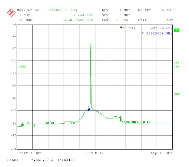
Marker 1: Calculated Field Strength (Restricted Band) = -70.44 + 16dBi antenna gain + 3 dB (MIMO) – 20 log (3 meters) + 104.77 = 43.79dB $\mu$ V/m Peak
