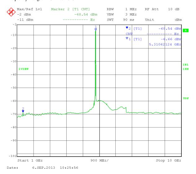
Marker 2: Calculated Field Strength (Restricted Band) = -68.54 + 16dBi antenna gain + 3 dB (MIMO) - 20 log (3 meters) + 104.77 = 46.1dB $\mu$ V/m Average
