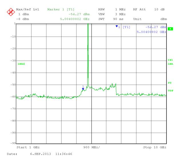
Marker 1: Calculated Field Strength (Restricted Band) = -54.27 + 16dBi antenna gain + 3 dB (MIMO) – 20 log (3 meters) + 104.77 = 59.96dB $\mu$ V/m Peak
