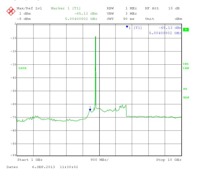
Marker 1: Calculated Field Strength (Restricted Band) = -65.13 + 16dBi antenna gain + 3 dB (MIMO) - 20 log (3 meters) + 104.77 = 49.1dB $\mu$ V/m Average
