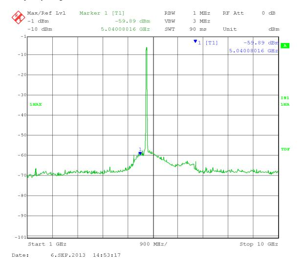
Marker 1: Calculated Field Strength (Restricted Band) = -59.89 + 16dBi antenna gain + 3 dB (MIMO) – 20 log (3 meters) + 104.77 = 54.34dB $\mu$ V/m Peak
