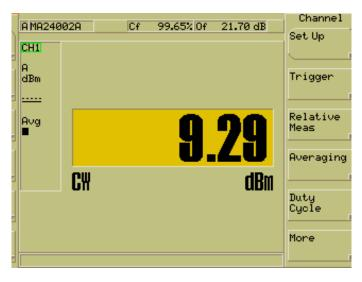
Ch 1: Maximum conducted output power = 11.27dBm + 3 dB (MIMO) = 14.27dBm < 15dBm = Pass
