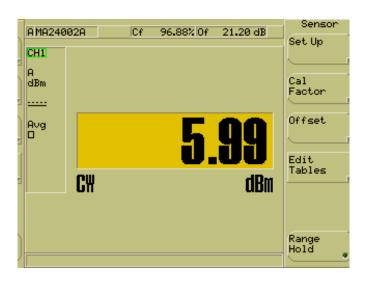
Ch 1: Maximum conducted output power = 6.28dBm + 3 dB (MIMO) = 9.28dBm < 15dBm = Pass
