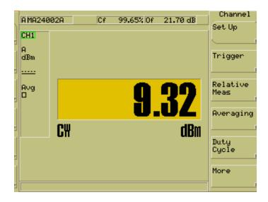
Ch 1: Maximum conducted output power = 11.87dBm + 3 dB (MIMO) = 14.87dBm < 15dBm = Pass
