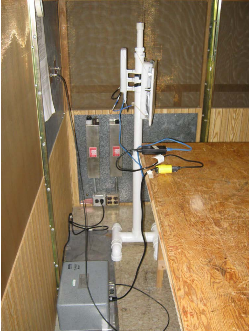
AC Line Conducted. Model C024045C008A with Panel Antenna
