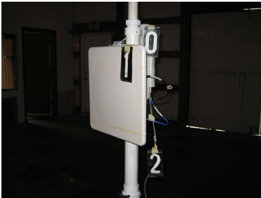
Radiated Emissions – Back - Below 1GHz with Panel Antenna
