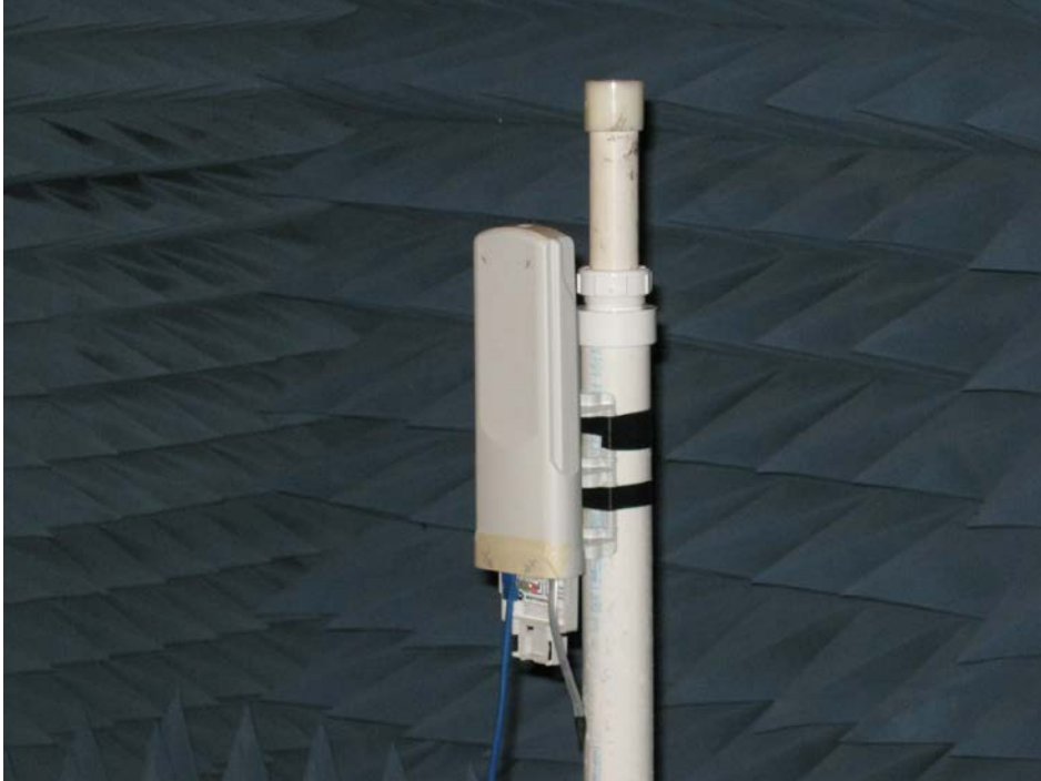
Radiated Emissions – 1 to 18GHz. Model C024045C004A with Patch Antenna
