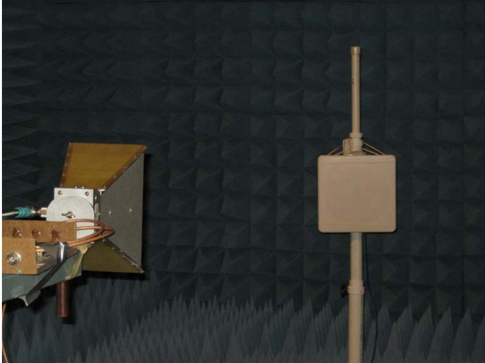
Radiated Emissions – 1 to 18GHz. Model C024045C008A with Panel Antenna
