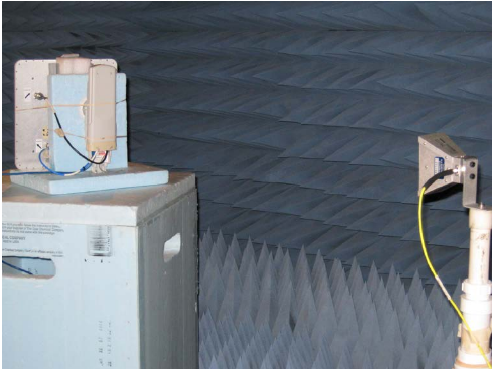
Radiated Emissions – above 18GHz. Model C024045C008A with Panel Antenna
