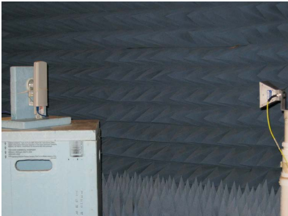
Radiated Emissions – above 18GHz. Model C024045C004A with Patch Antenna
