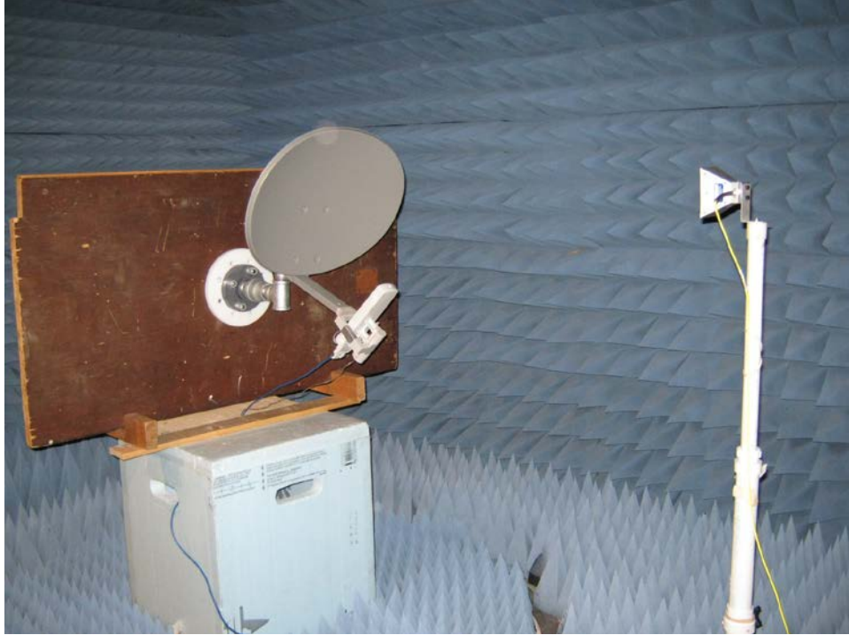
Radiated Emissions – above 18GHz. Model C024045C004A with Dish Antenna
