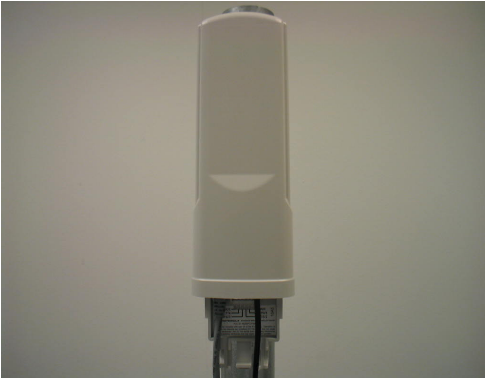
900MHz Canopy Radio Mounted in Chassis – Integrated Assembly
