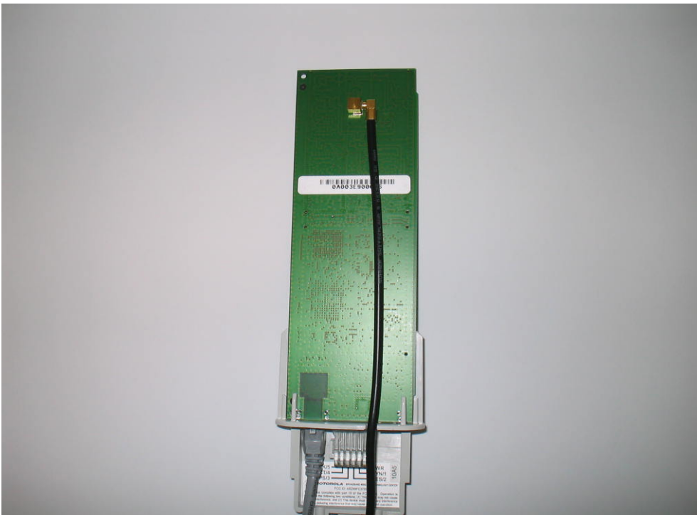
900MHz Canopy Radio Mounted in Chassis – RF Connector View
