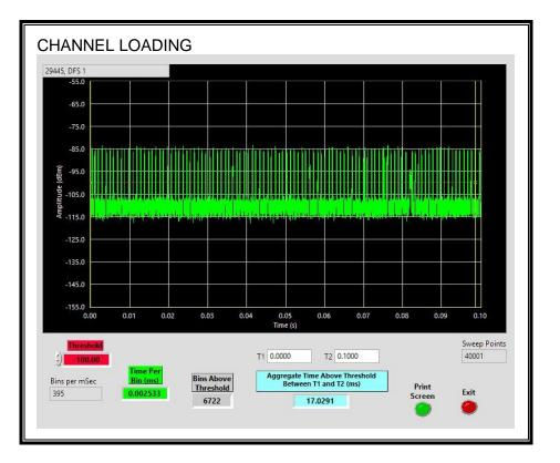
The level of traffic loading on the channel by the EUT is 17.029%
