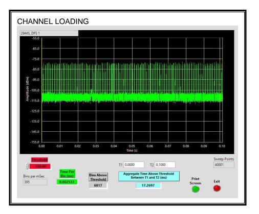
The level of traffic loading on the channel by the EUT is 17.26%
