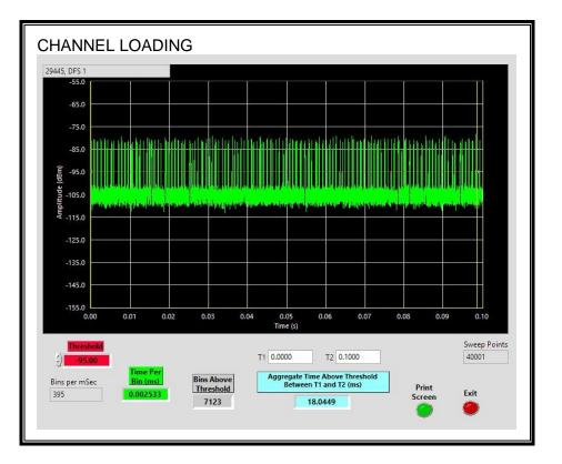
The level of traffic loading on the channel by the EUT is 18.04%
