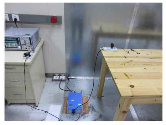
FCC RADIATED EMISSION TEST SETUP
