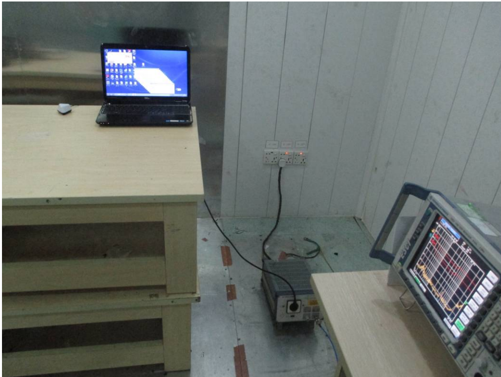
FCC RADIATED EMISSION TEST SETUP
