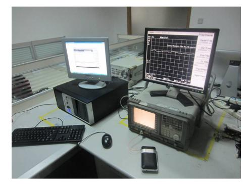
CONDUCTED EMISSION TEST SETUP
