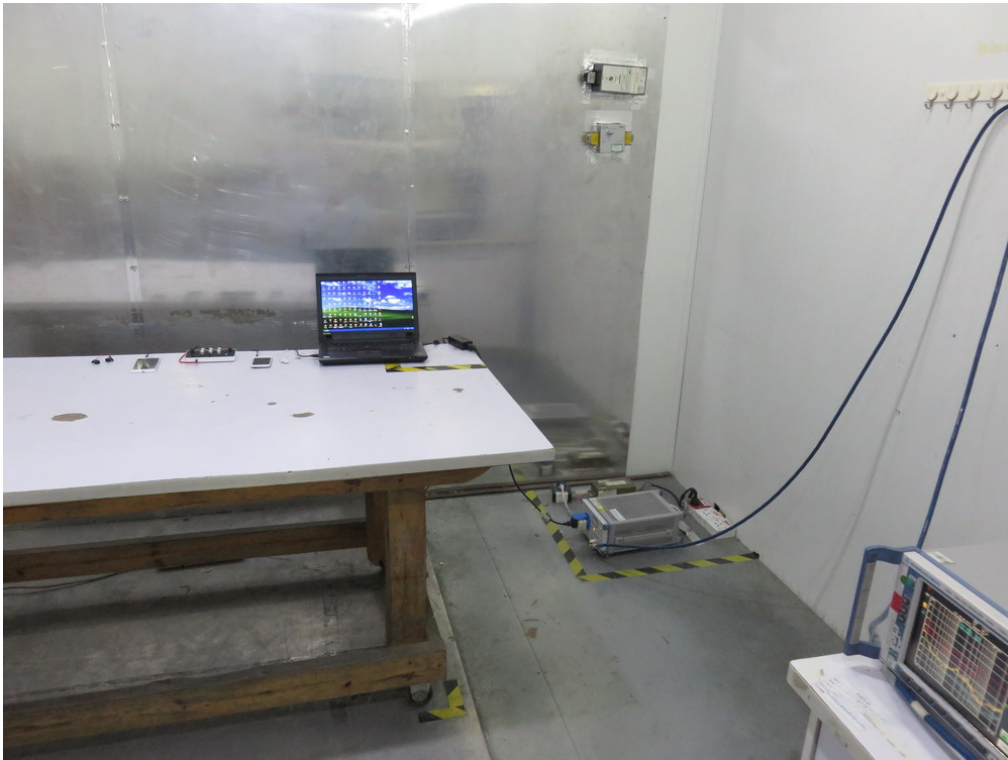
FCC RADIATED EMISSION TEST SETUP
