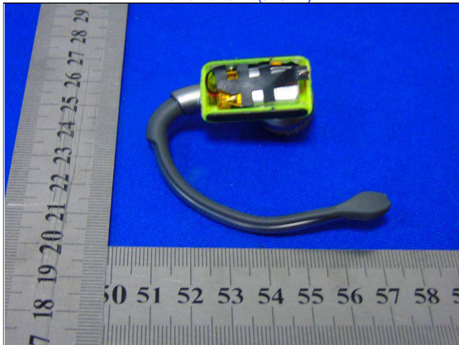
The new antenna(3M9471)
