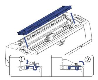
5) Insert/remove the ribbon fabric in-between the print head and ribbon mask by squeezing the outside wings of the Ribbon Guide, as shown, to position and secure the ribbon onto the print head.
