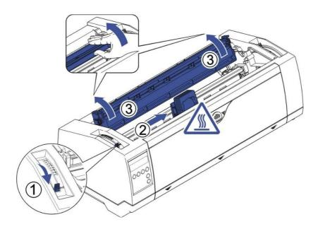
4) Insert the ribbon cartridge till it is tightly locked in position.
