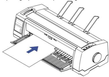
6) Press the load key to feed the paper to the correct print position, automatically. The printer clears the Paper End condition and goes into the ready or online state.
