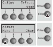
Select the Setup mode by pressing the Setup key.
