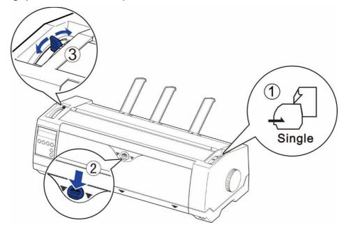
4) It is recommended to align the left paper guide exactly to the mark > I <. This marks the left edge of the stationery. Slide the right guide to the position of the right edge of the stationery.
