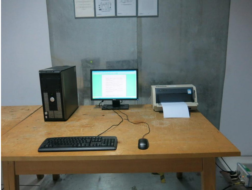
Photograph 2: Set-up for Radiated Emissions of below 1GHz
