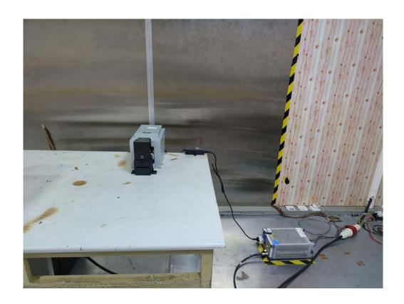
M/N: DC-2300 Radiated Test (Below 30MHz)
