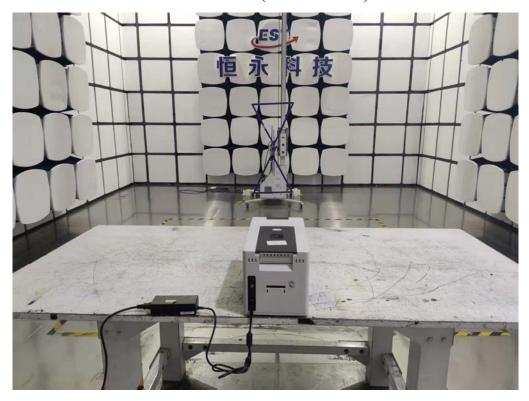
M/N: KT-200 Radiated Test (Above 30MHz)
