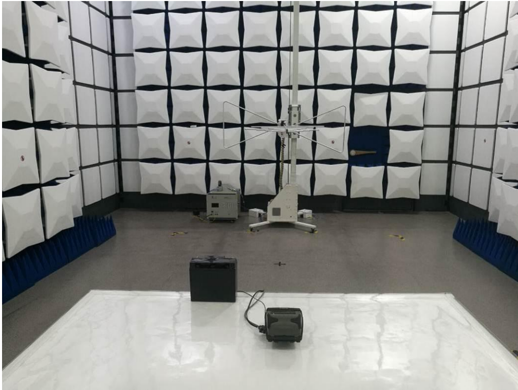
FCC RADIATED EMISSION TEST SETUP
