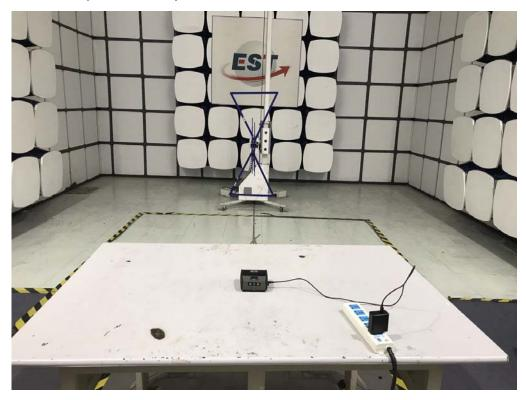
Radiated Test (Above 1GHz)
