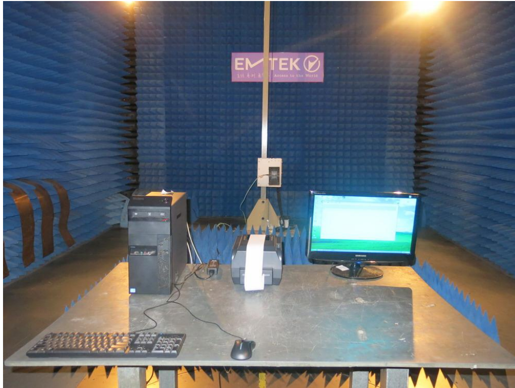
Photograph 3: Set-up for Radiated Emissions of 1 - 2GHz
