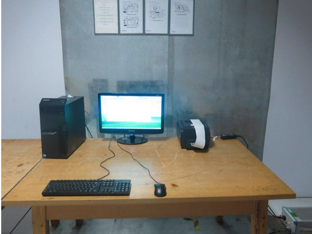
Photograph 2: Set-up for Radiated Emissions of below 1GHz
