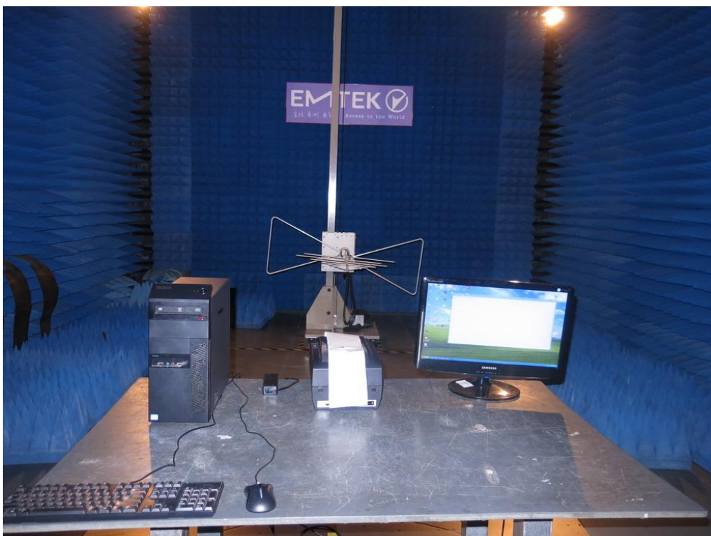
Photograph 2: Set-up for Radiated Emissions of below 1GHz
