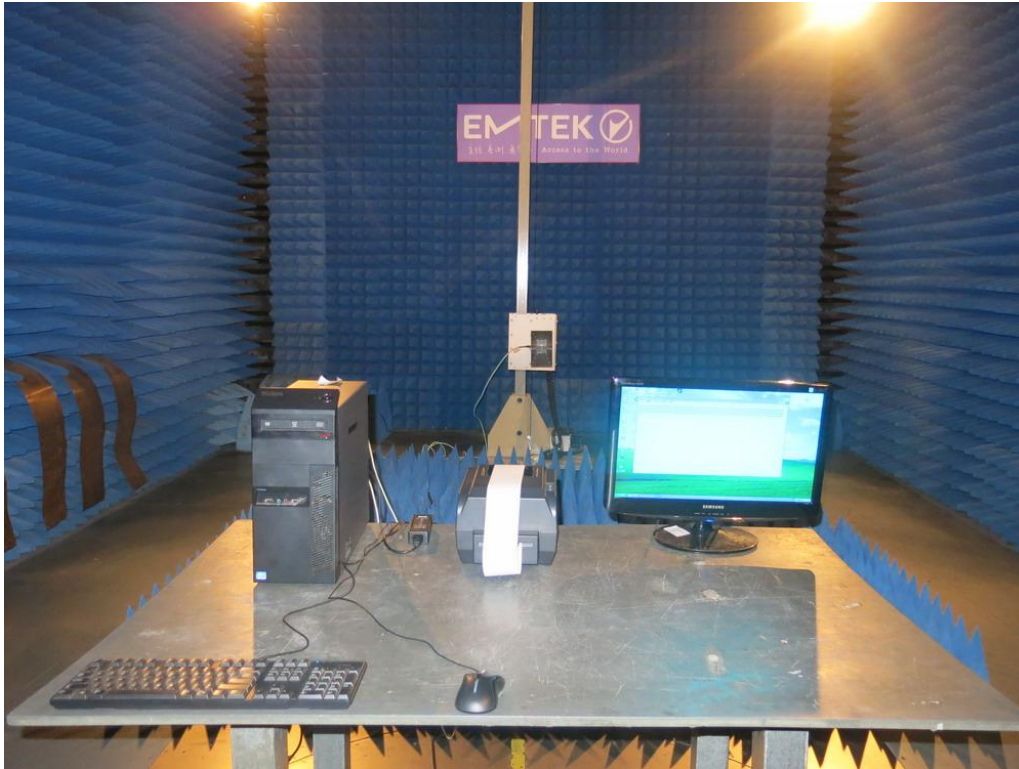
Photograph 3: Set-up for Radiated Emissions of 1 - 2GHz
