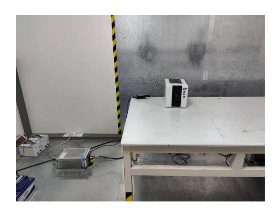
Radiated Test (Below 30MHz)
