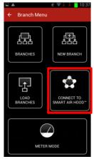
To connect to the SMART Air Hood<sup>TM</sup>, tap the SEARCH button to locate it, and tap on the empty square of the found SMART Air Hood<sup>TM</sup> device.
