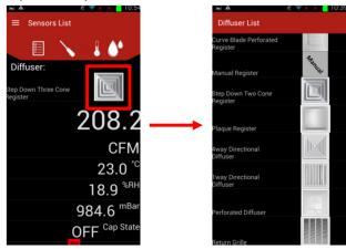
Tap on the appropriate icon to select that diffuser style, which in this example is the *Plaque Register*. Now the Plaque Register diffuser style is selected assuring accurate flow measurements.
