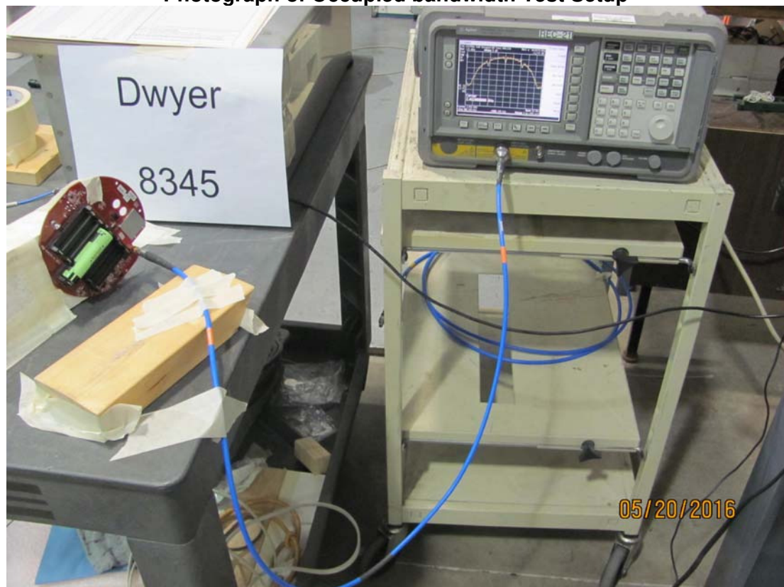
Photograph of Occupied bandwidth Test Setup
