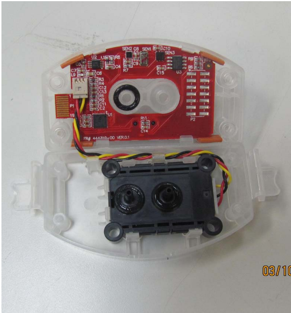
Photograph of Sensor: Case Open
