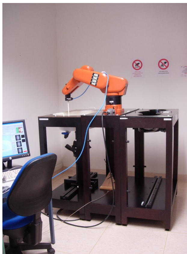
Picture A - SAR Dosimetric Assessment System
