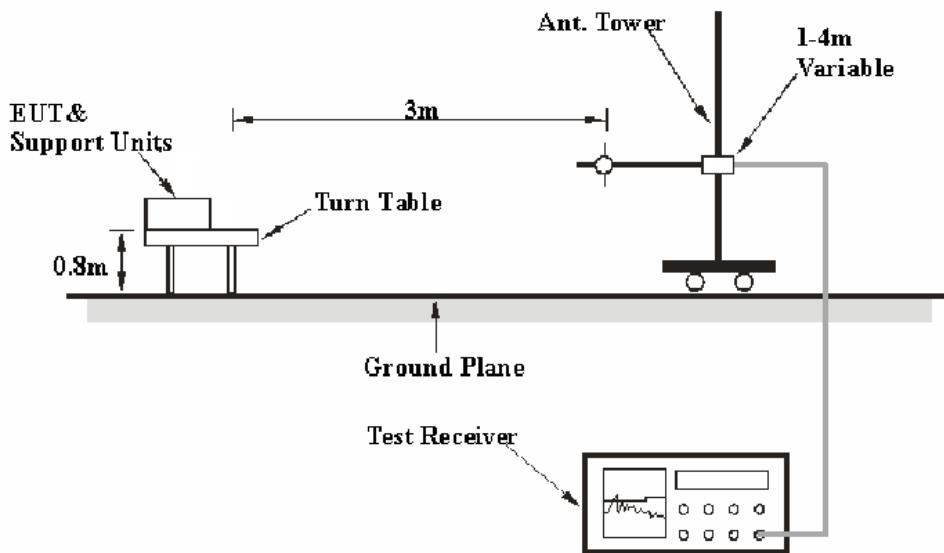
The radiated emission tests were performed in the 3 meters chamber B test site, using the setup accordance with the ANSI C63.4-2009. The specification used was the FCC Part 15 Class B limits.
