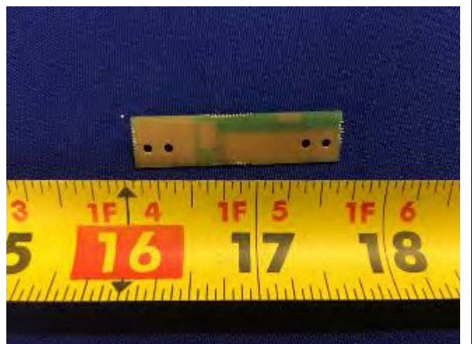
Antenna - Bottom View
