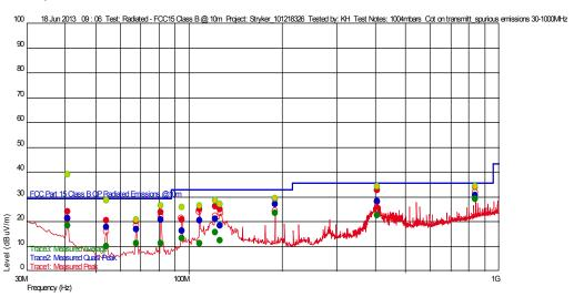
Measured Peak Value Swept Peak Data Measured Quasi Peak Value Swept Quasi Peak Data Measured Average Value Swept Average Data Maximum Value of Mast and Turntable
