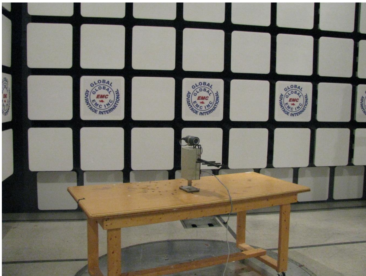
Figure 1 – Radiated emission setup
