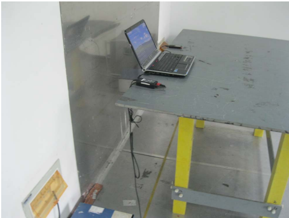
Conducted Emissions Test Setup - Side View
