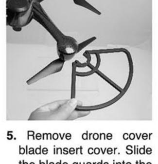
the blade guards into the drone and secure using screws.
