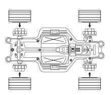
Install your wheels to chassis until you hear a "click". Remove wheels by pulling straight out.
