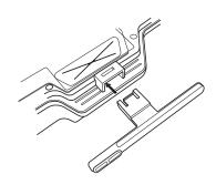
Snap side exhaust pipe or side step by snapping into side of chassis until you hear a "click". (reversible)
