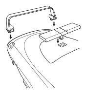
Install rear spoiler, roof light and hood scoop by snapping onto body shell. A "click" sound can be heard when parts are fully inserted.
