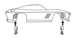
Install chassis mounts to the shell.
