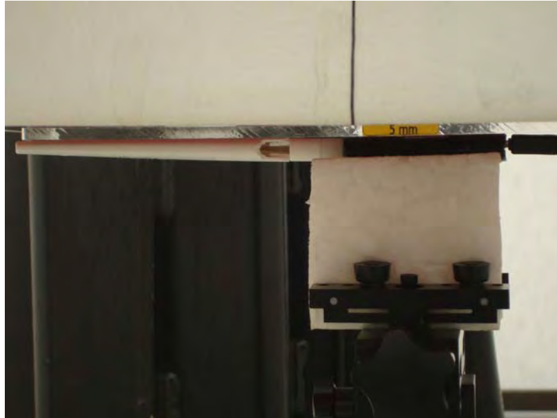
Figure 1. Body SAR Test Setup (Flat Section)_ Horizontal Up with USB Cable_antenna straight mode
