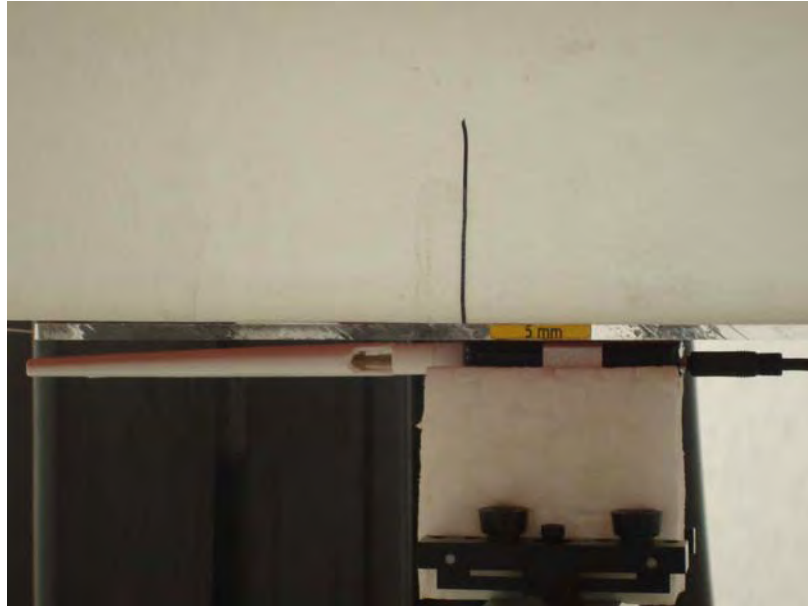
Figure 2. Body SAR Test Setup (Flat Section)_ Horizontal Down with USB Cable_antenna straight mode
