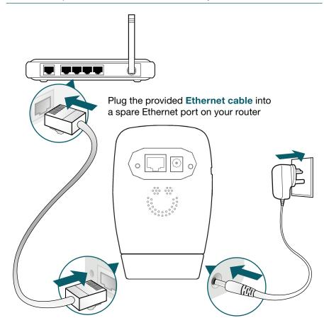
Plug the other end of **Ethernet** cable into the Ethernet port on the back of the Babelens Video Monitor
