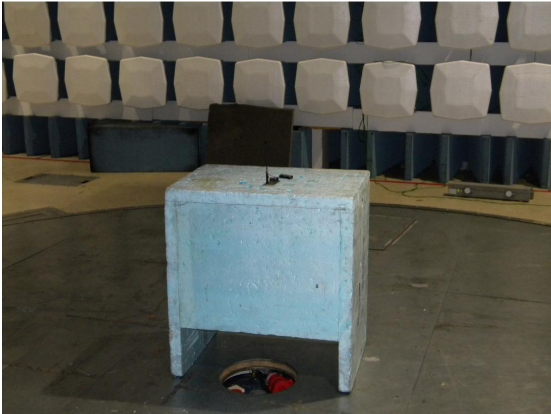
Photograph 1, Radiated emissions test setup.
