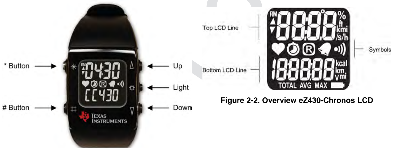
Figure 2-1. eZ430-Chronos Watch Push Buttons
