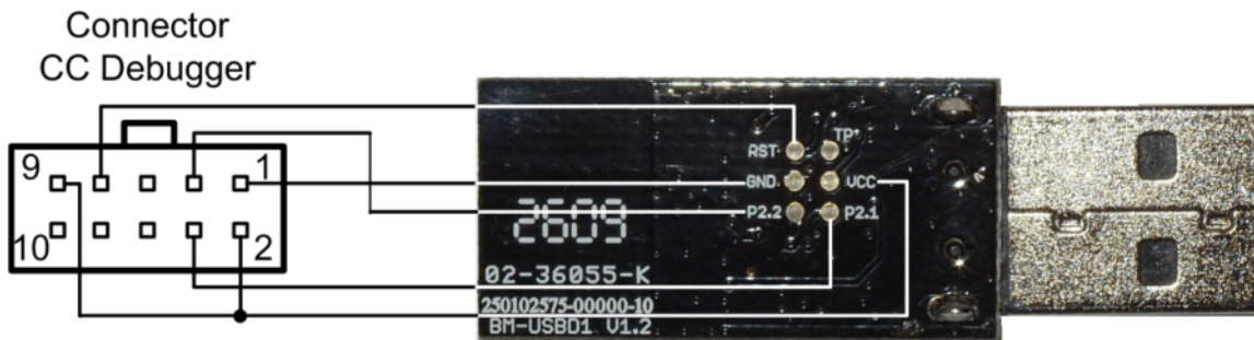
Figure 3-16. eZ430-Chronos RF Access Point Connection to CC Debugger
