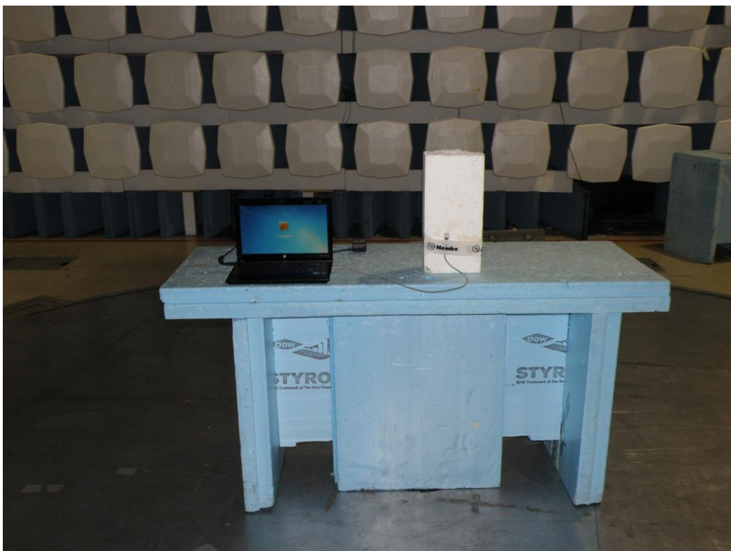
Photograph 2, Spurious emissions test setup
