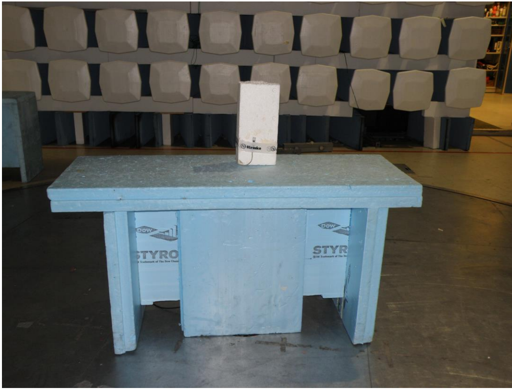
Photograph 1, Radiated max power test setup
