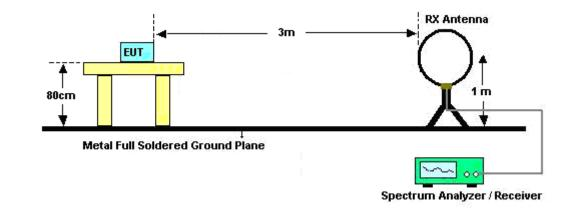
For radiated emissions from 30MHz to 1GHz
