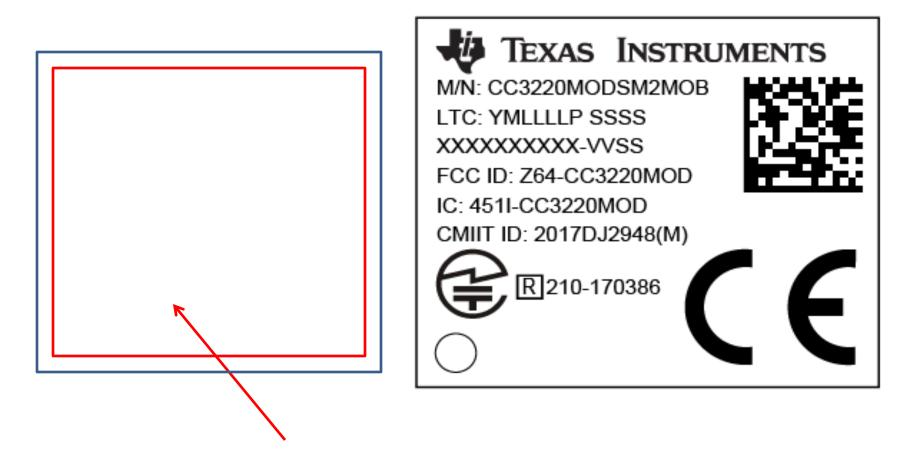
Information is laser etched onto the metal can of the module
