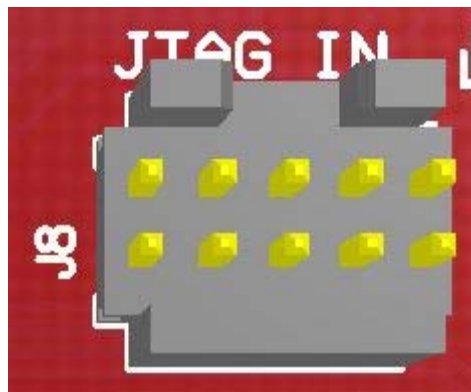
Figure 2-4: JTAG Input Connector for Using External Emulator
