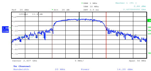
Figure 8.4-3: Output power on 802.11n, sample plot
