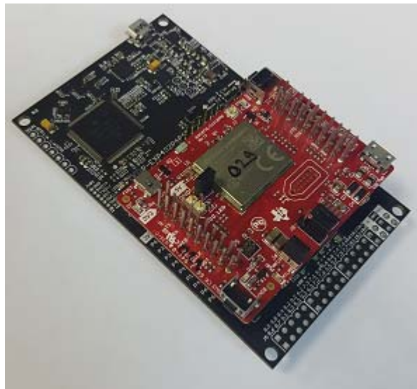
Figure 7-9: BOOSTXL-CC3120MOD Connected to MSP432 LaunchPad
