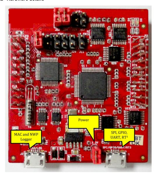
The board has two FTDI ICs to enumerate multiple COM and D2XX ports. The details of the ports are given below
