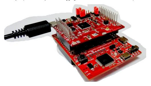
FIGURE 3: BOOSTER PACK CONNECTED TO TIVA LAUNCHPAD
