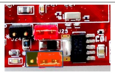
FIGURE 4: JUMPER SETTINGS WHEN USED WITH LAUNCHPAD
