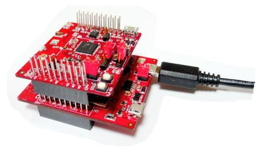
FIGURE 2: PC CONNECTION USING FTDI
