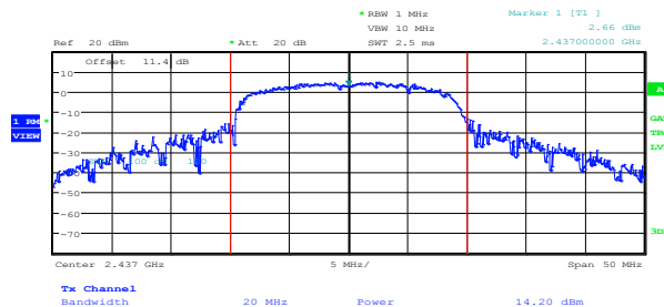
Figure 8.4-3: Output power on 802.11n, sample plot
