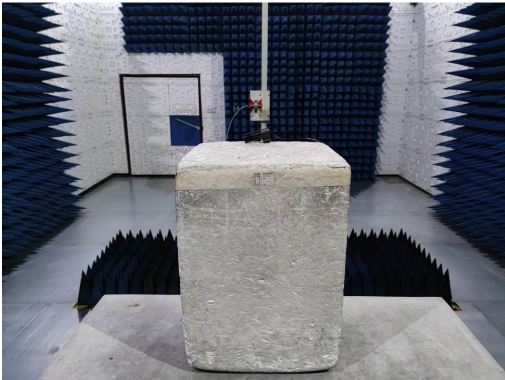
RADIATED EMISSION TEST SETUP ABOVE 1GHz
