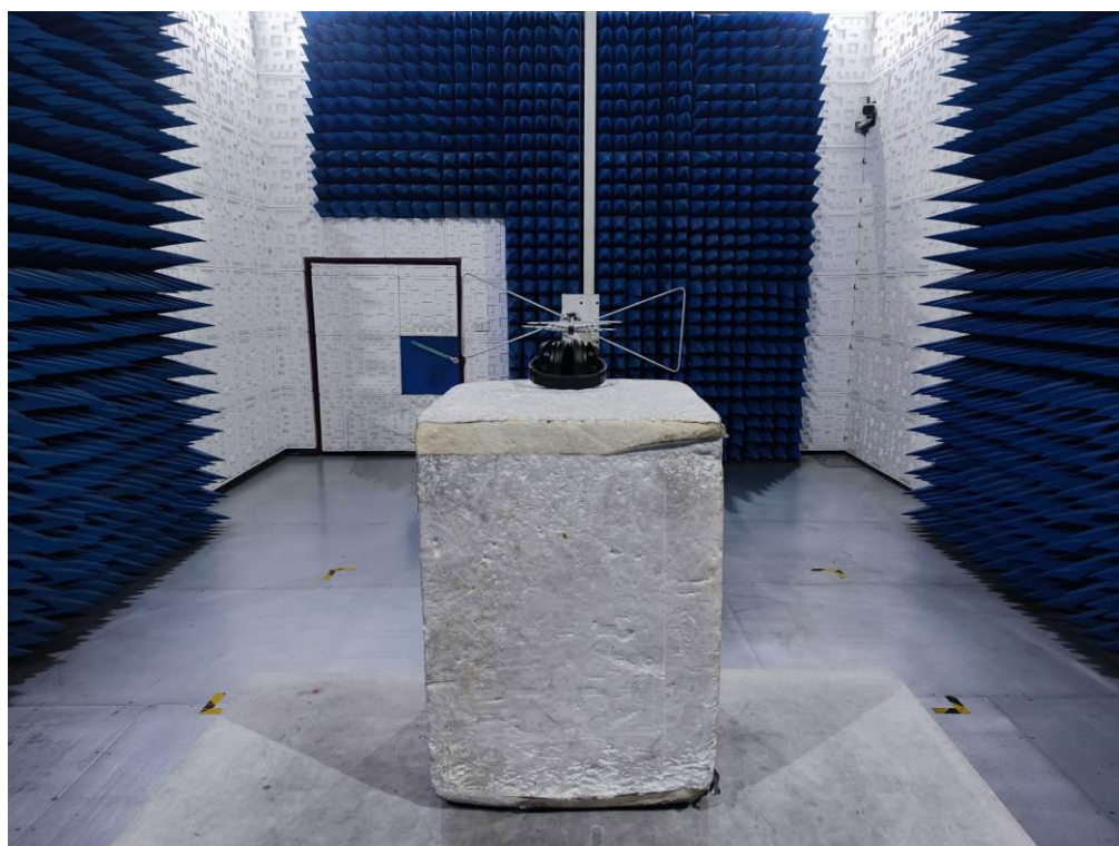
RADIATED EMISSION TEST SETUP ABOVE 1GHz
