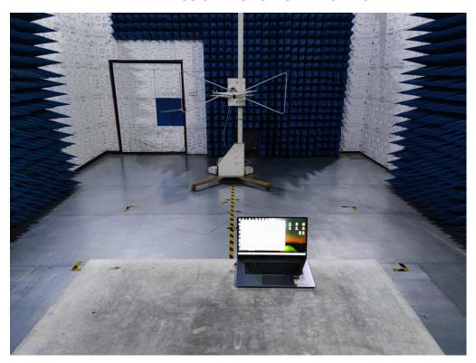
RADIATED EMISSION TEST SETUP ABOVE 1GHz
