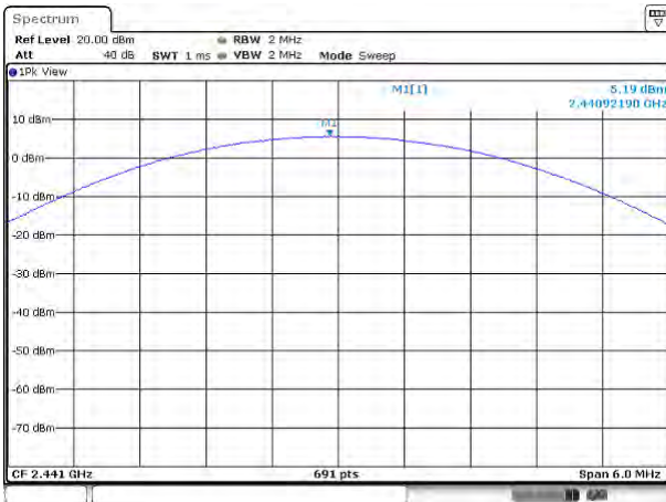
Peak output Power plot on channel 39 (3Mbps)
