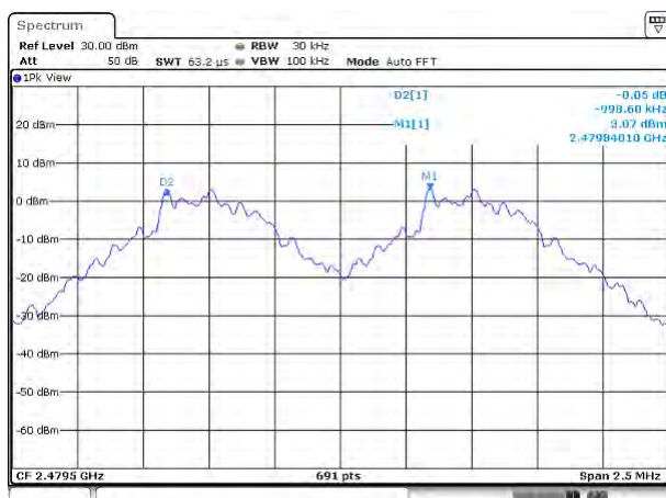
(1Mbps) Channel Separation plot on channel 77-78
