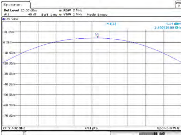
Peak output Power plot on channel 39 (1Mbps)
