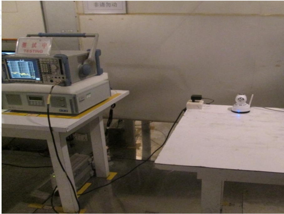
TEST SETUP OF CONDUCTED EMISSION
