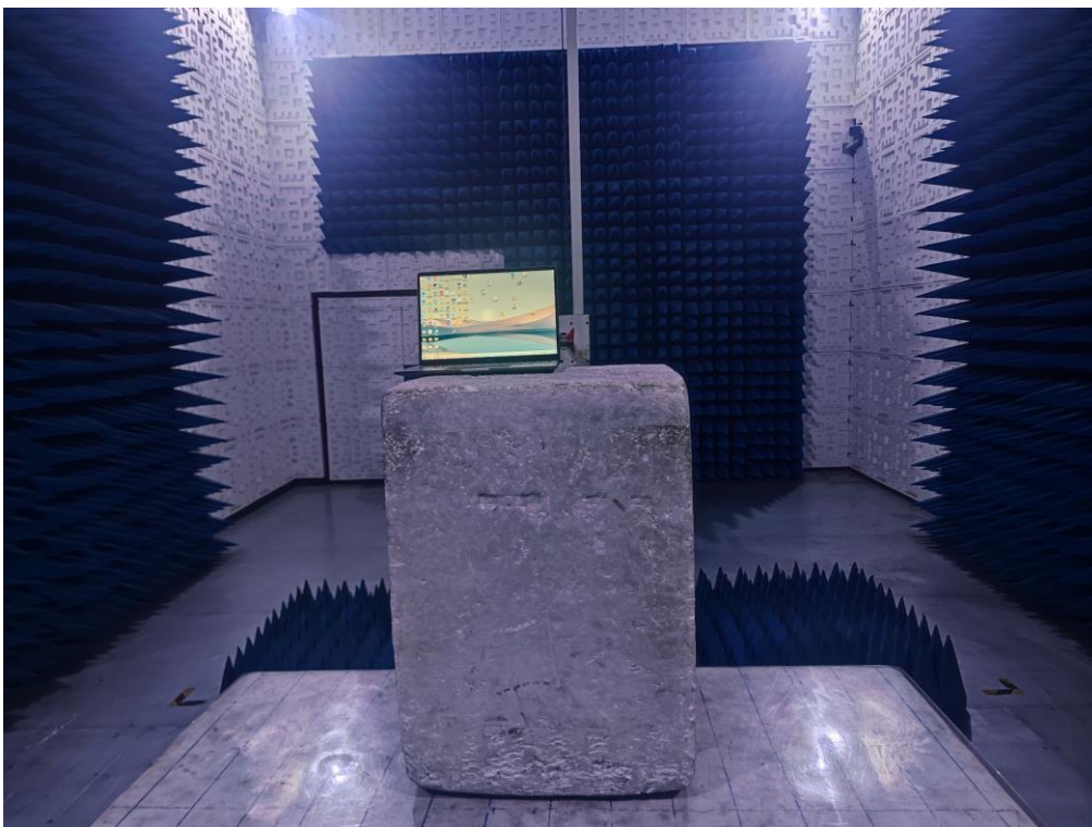
RADIATED EMISSION TEST SETUP ABOVE 1GHz
