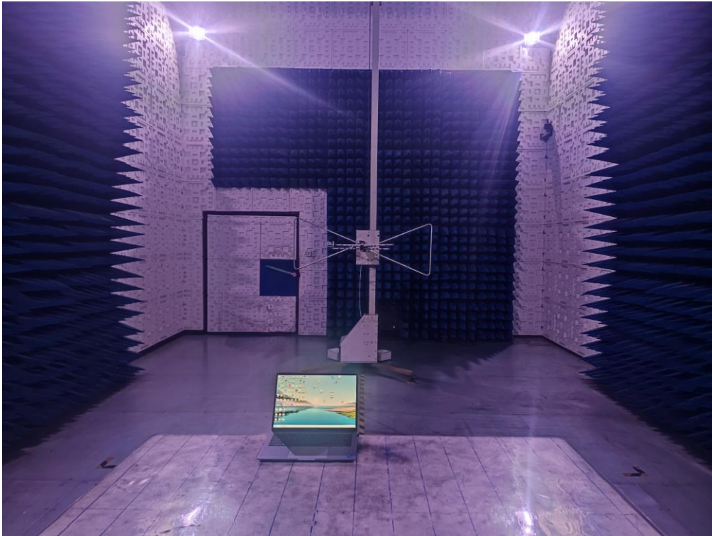
RADIATED EMISSION TEST SETUP ABOVE 1GHz
